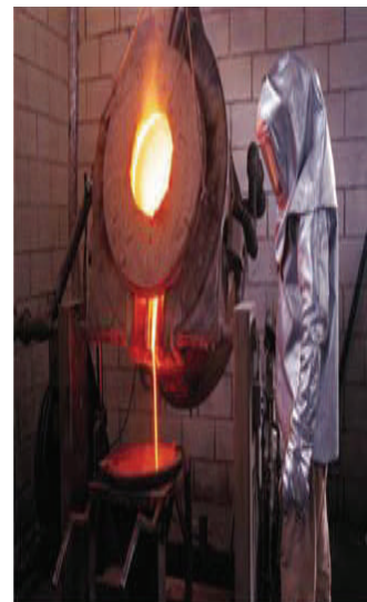
Molten metal is a burn hazard and inhalational hazard.
